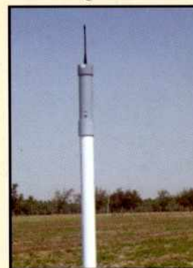
Wireless Sensor Module for Soil Moisture, EC and Temperature Measurement
